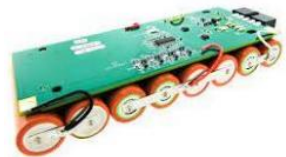
Battery Management System
